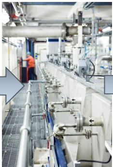
Solvent extract Morphine in belt extractor
